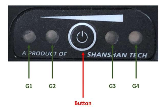
Note: The button is only for LED display, not the power button.
